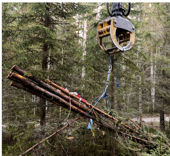
Figure 2. Scaling of the tree bunches by means of a dynamometer and a forwarder crane.
