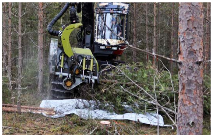
Figure 1. The “MAMA” head used in field trials for processing a bunch of trees on a blanket to collect the scraped-off biomass.
