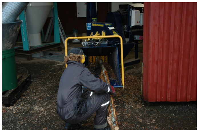
Figure 1. Manual feeding of a small log during the chipping experiment.
