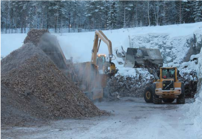
Figure 2. Stump crushing at a terminal with crane loader and front-end loader.
