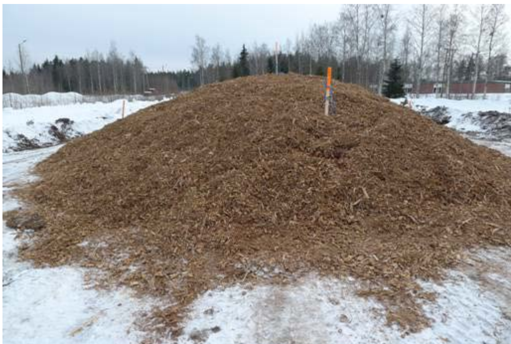
Figure 2. Pile of pulp mill birch bark at UPM Pietarsaari mill. The sample for the analysis of suberin was taken right after the wet debarking. The pile in this photo was constructed for the storage experiment where changes in chemical and physical properties of the bark are monitored
