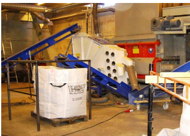
Fig 2. Gravimetric separator for commercial use sieving
