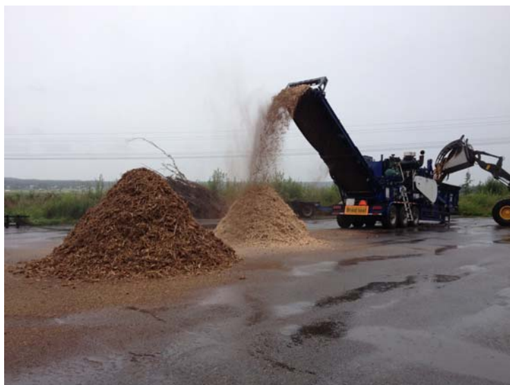
Fig 1. Crushing of stump samples (left) and chipper used for the reduction of particle size, \varnothing 8-12 mm, of the small tree sample (right).
