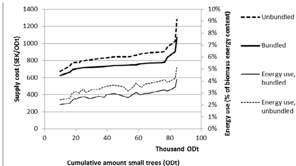
**Figure 1.** Supply cost and energy use for whole trees from energy thinnings with and without bundling, based on the case study of Örnsköldsvik. Chipping at terminal and delivery to industry is included.
