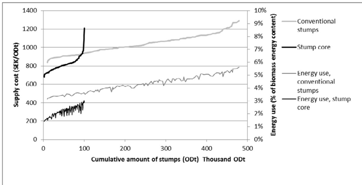
**Figure 1.** Supply cost for stump core harvest compared to supply cost for conventional stump harvesting, based on the case study of Örnsköldsvik. Chipping and delivery to industry is included.
