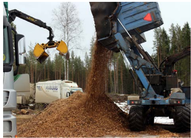
Figure 3. Machine system (forwarder-mounted chipper and chip-truck with self-loading crane) for working at the forest roadside and delivering chips to end-user or terminal.
