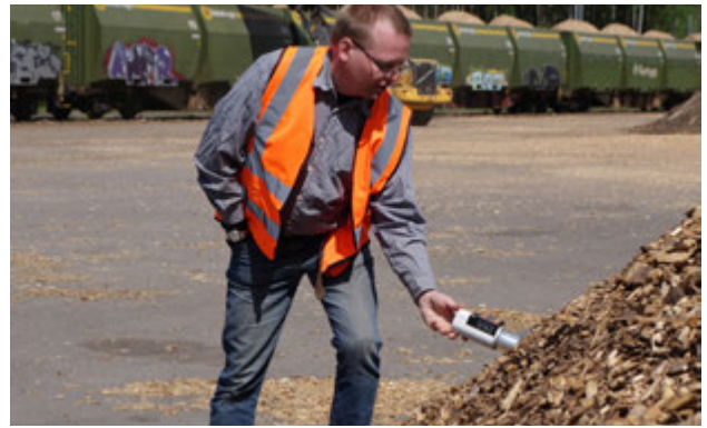
Measuring moisture content in the field. Leif Westerlund, SLU
