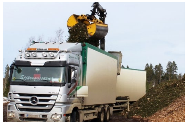
Figure 5. Operation of the modelled self-loading chip-trucks.
