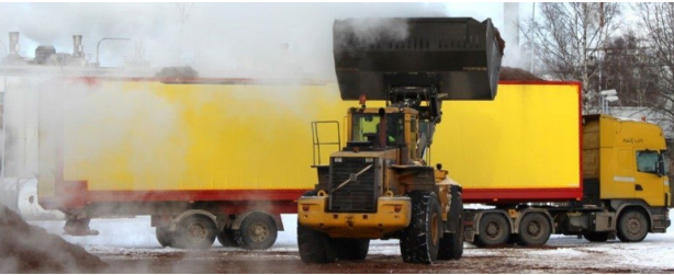
Figure 7. Operation of the modelled wheel-loader and shuttle chip-truck in the terminal.
