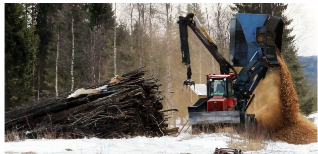
Figure 4. Operation of the modelled forwarder-mounted chipper.
