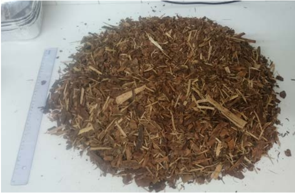
Figure 2. Dried, uncomminuted, bark used in the study. The scale in the figure is 40 cm long.
