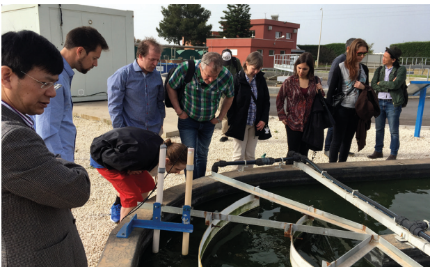
The pilot scale cultivation unit consists of six raceway's of each 32 m 2 .
