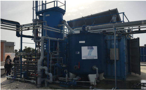
Harvesting of microalgae using nanobubbles.
