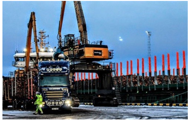
Figure 8. Multidocker CH65 port material handlers unloading pulpwood from the boat.
