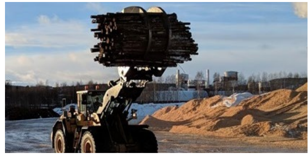
Figure 4. Volvo 180G wheel loader equipped with log grapple at the mill log yard.
