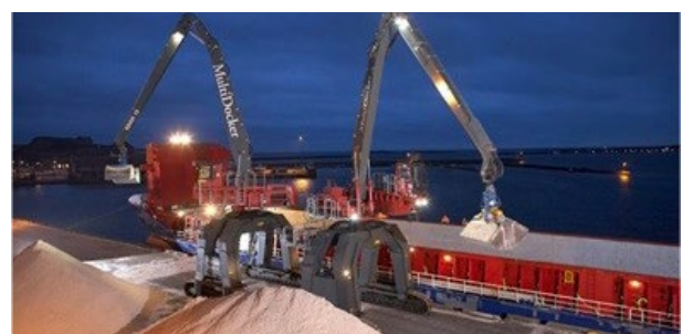
Figure 2. Multidocker material handler at the port
