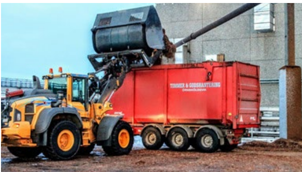
Figure 1. Volvo L120H loading bark into the trailer
