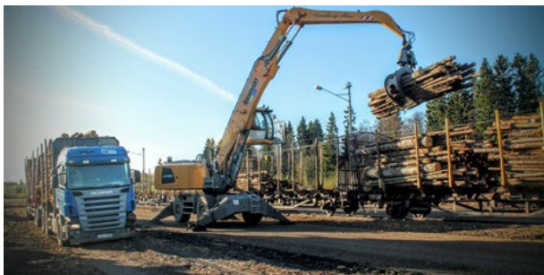
Figure 6. Liebherr LH50 material handler at the feed-in pulp log terminal.
