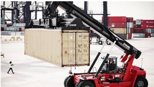
Figure 3. Reach stacker for container handling
