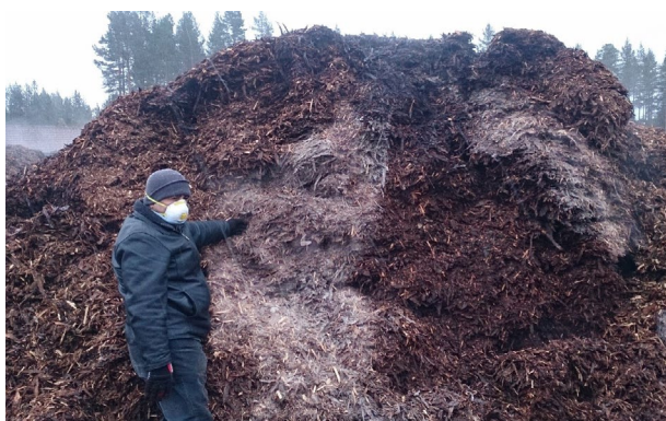
Fig. 2. Massive microbial infection during storage of bark in an uncovered pile.
