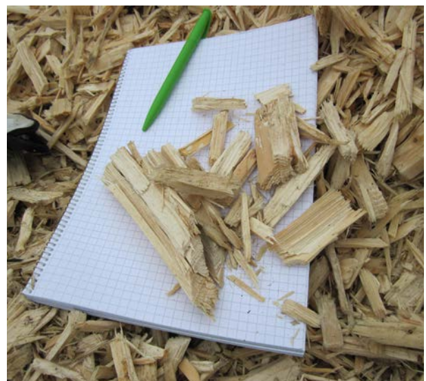
Figure 1. Chips of small diameter roundwood produced with a mobile chipper.
