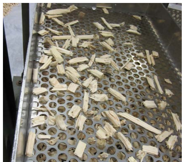
Figure 3. Wood chips on a perforated screen tray of SCAN CM 40-01.
