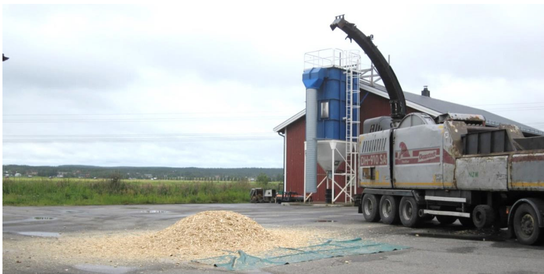
Figure 2. The mobile chipper used in the study produced approximately three cubic meters of chips.
