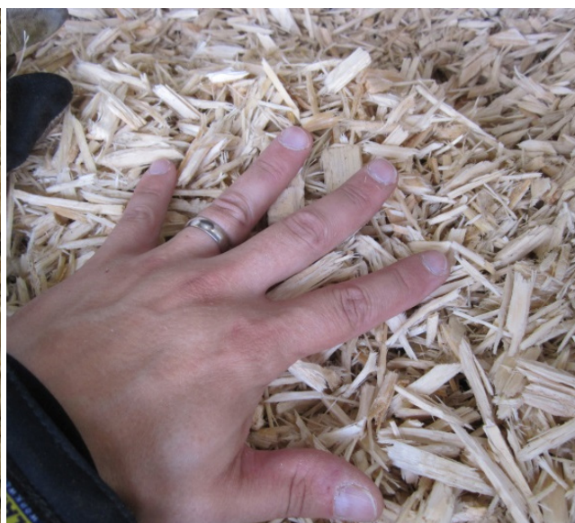
Figure 3. Wood particles chipped using the mobile Doppstadt DH-910 SA-drum chipper (left) and these particles comminuted using the Lindner Micromat 2000-shredder (right).
