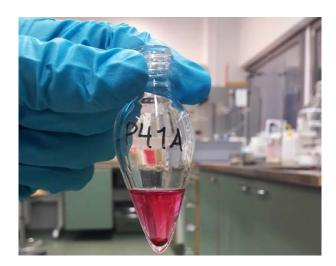
For acid hydrolysis the carbohydrates in the bark samples were hydrolyzed and solubilized by sulfuric acid. The acid-insoluble lignin (Klason lignin) was filtered off, dried and weighed (TAPPI T 222 om-02). The acid-soluble lignin was determined from the filtrate via UV/ Vis-spectrophotometer. at 215 and 280 nm.
