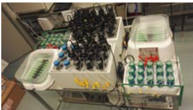
Figure 2. Two AMPTS II-units by Bioprocess Control at Technobothnia in Vasa, Finland. They are used to find out the BMP of substrates and thus the pretreatment effect.
