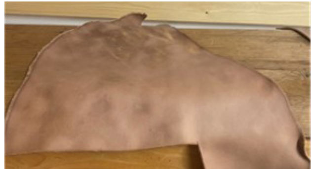
Figure 5. A leather from Kokkolan Nahka treated naturally using tannins from spruce logging residues.
